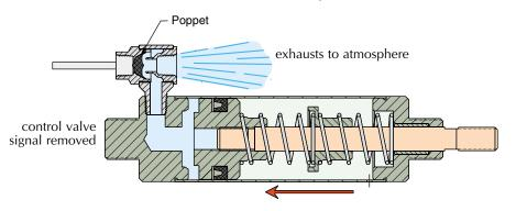
In a typical application the exhaust valve is installed in the inlet of a spring return or double acting pneumatic cylinder.
